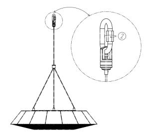
Step 3:Tighten the nut in direction of rotation arrow.
