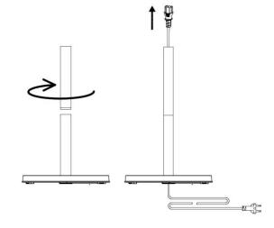
Step 3: Connect the top tube with middle tube by screwing them together (as same as Step2).Place the power cord plug through the base, bottom tube and middle tube and top tube.
