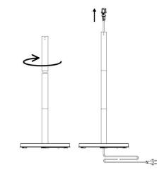
Step 4: Place the power cord plug through the base , bottom tube, middle tube and top tube. Connect the power cord plug to the socket in the heater head.
