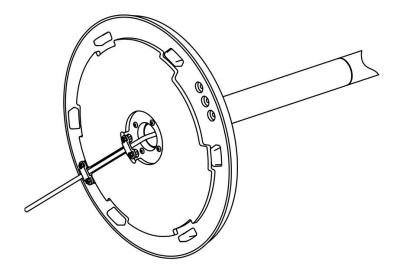
Step 7: Fix the heater on the floor. Bore three holes in the floor, fix the heater by three wedge bolts on the floor tightening the screws by spanner.
