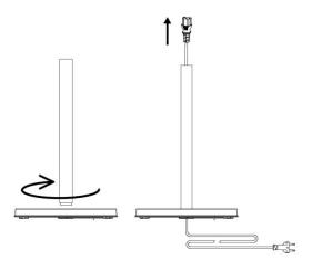
Step 2: Connect the middle tube with bottom tube by screwing them together.Place the power cord plug through the base, bottom tube and middle tube.
